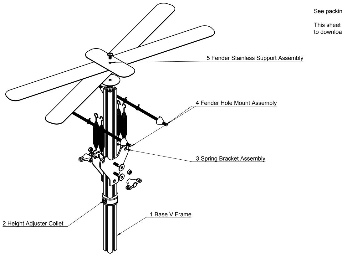
VAX-MC-FNDR VsionAir Fender Jig Assembly See packing list for parts breakdown.
